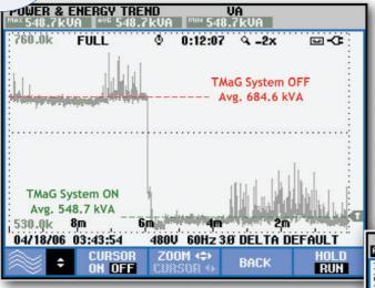
Below are actual meter display results of a PureMon1cs™ TMaG System™ that shows dramatically improved distribution system efficiency and reduced power demand on a 1000kVA main distribution transformer.
