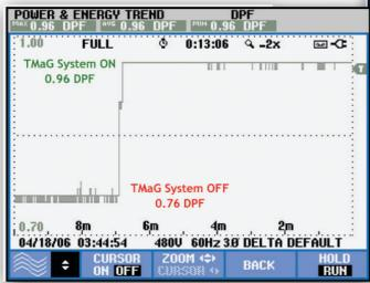
NOTE: Data collected using a Fluke 434 Power Quality Analyzer. Results (as shown above) are application specific and based upon distribution system efficiency and facility load profile.
